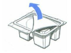
Remove the protective material from the BJ cartridge.
